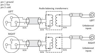
fig. 10: Balanced - Unbalanced wiring using transformer
