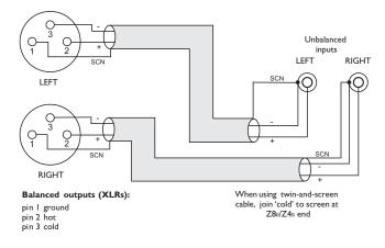
$\textit{fig. I 2:} \ Balanced - Unbalanced \ input \ \#2$
