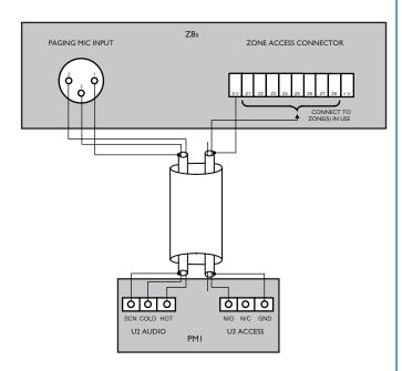
fig. 19: PMI - Z8II wiring connections
