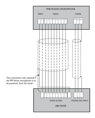
fig. 18: PM8 - Z811 wiring connections
