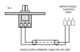
fig. 19: RL-I control wiring
