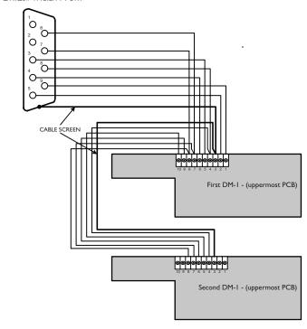
fig.23: Connecting multiple DM-I plates
