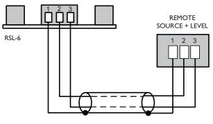
REMOTE SOURCE & LEVEL CONTROL WIRING
