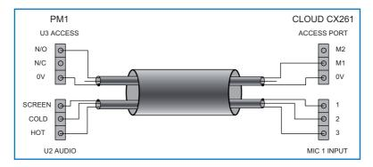
In the example, 2-pair cable is employed, with separate screened twin-and-screen cores for the Audio and Access connectors. The PMI's audio output is wired pin-topin to the MIC 1 INPUT connector on the CX261. The access connector is wired to the CX261's Access Port, the ground terminal being connected to 0V on the host via the cable screen and the N/O terminal to M1.
