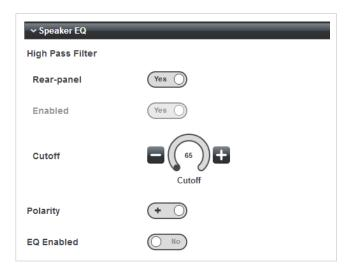
Setting Rear-panel to No disables the DIP switches and control of the high-pass filter is now only from the browser. However, the filter itself may still be taken out of circuit altogether by setting the Enabled switch to No. This restores the amplifier channel's full frequency response.
