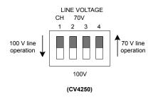
The voltage may be set independently for each channel. Set the switch UP for 70 V-line operation and DOWN for 100 V-line operation.
