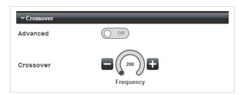
With Advanced set to Off, a default crossover is implemented, adjusted by the Frequency control: the crossover type is a Linkwitz-Riley filter with a slope of 24 dB/octave. The range of adjustment is the full audio range of 20 Hz to 20 kHz. Signal content above the crossover frequency will be routed to the HF Speaker channel (in this example, Channel 3) and content below the crossover frequency to the LF Speaker channel (in this example, Channel 4).
