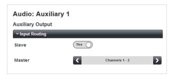
Auxiliary Outputs are by default mono. When one is slaved to a stereo pair of channels, its source becomes a mono sum of the signals in the two channels. Alternative, mono amplifier channels will be available as sources via the Master selector as single channels in the normal way. Source selection for Auxiliary Outputs when they are not in Slave mode is unchanged: any Line Input (or off) may be selected.
