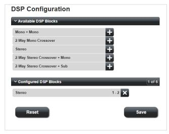
DSP blocks will be added to the Configured DSP Blocks tab in ascending numerical order. The above screenshot indicates that Channels 1 and 2 will form a stereo pair. If this is the only stereo block required and the other amplifier channels are to remain mono, click the + to the right of the Mono + Mono block as many times as necessary to fill the available DSP slots (the number varies with model):
