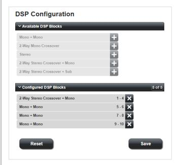
This configuration actually only requires three amplifier channels to be configured for the crossover itself: the fourth channel remains mono and independent. It is included in the DSP block allocation, however, because DSP blocks can only be allocated in odd/even pairs. The result can be seen in the drop-down menu:
