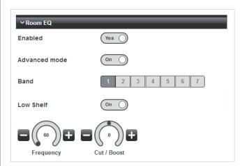
The Room EQ is now reconfigured as a seven band parametric equaliser, with peak/shelf switching on the highest and lowest bands. The Band buttons assign the rotary controls to each frequency band in turn: all bands have the same frequency range of 20 Hz to 20 kHz, adjusted by the Frequency control. However the seven default centre frequencies are 60 Hz, 250 Hz, 1 kHz, 2 kHz, 4 kHz, 8 kHz and 16 kHz, which will be suitable for most installations. The Cut / Boost control has a range of +/-12 dB.
