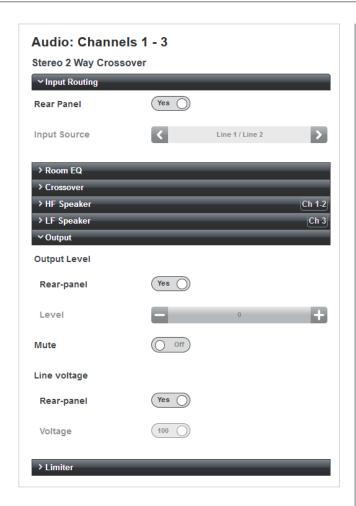
The status of the three channels is confirmed at the top of the page. The page has the same seven tabs as the 2-Way Mono Crossover Audio page. Note however, that the HF Speaker tab is now annotated Ch 1-2 and the LF Speaker tab Ch 3, indicating that (in this example), these are how the channels are deployed.
