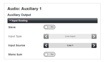
Input Source – the default source is Input 1 for Auxiliary 1 and Input 2 for Auxiliary 2. Click the < and > buttons to select an alternative input. Every input is available to either Auxiliary Output. Clicking > when the highest-numbered input is showing selects off, which removes all input sources from the auxiliary channel. Once enabled, this control will also be displayed on the Overview page.
