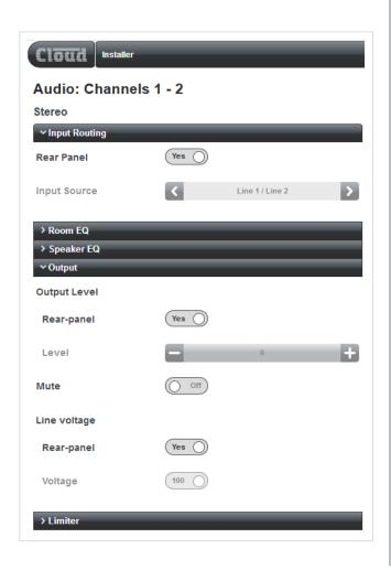
Compare this with the corresponding page for a mono channel (see page 21). The only differences lie in the Input Routing tab: the Input Source selector now presents odd/even pairs of Line Inputs. Also note the Mono Sum switch is not present on stereo channels (as it would defeat the purpose of a stereo channel):
