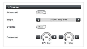
This permits a greater degree of control in tailoring the response of the crossover. Both filter controls have the full audio range of 20 Hz to 20 kHz, and thus the turnover frequencies of each filter section may be adjusted to be as close together or as far apart as wished, the variation determining the flatness of overall frequency response in the crossover region. Again, loudspeaker manufacturers will generally offer recommendations for particular speaker types.
