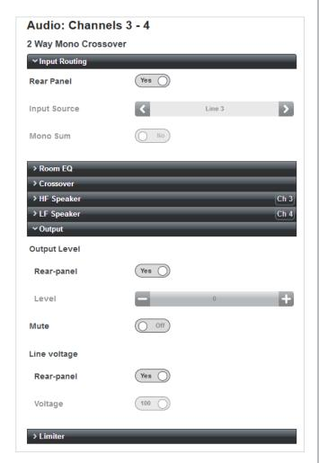
Note that the revised status of Channels 3 and 4-2 Way Mono Crossover-is confirmed at the top of the Audio page. The page is now divided into seven tabs: Input Routing, Room EQ, Crossover, HF Speaker, LF Speaker, Output and Limiter. The facilities on the Input Routing, Room EQ, Output and Limiter tabs are identical to those on a standard mono or stereo channel; the Speaker EQ tab is replaced by three tabs related to bi-amped operation.
