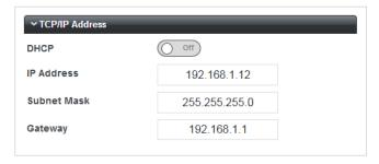
The current IP Address, Subnet Mask, Gateway address and Unit Name are confirmed. If DHCP is set to On, the values in IP Address, Subnet Mask and Gateway are set automatically and the fields greyed out. If assigning these values (with DHCP set to Off), ensure that a suitable, reserved static IP address is used. This may require consultation with the network administrator.
