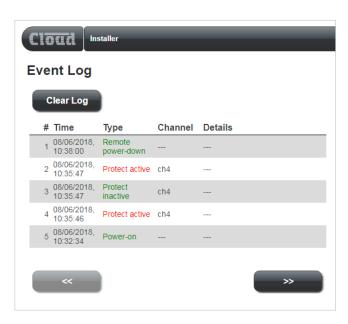
The amplifier can maintain a log of critical events. This can be viewed to check whether amplifier fault conditions have given rise to operational problems.
