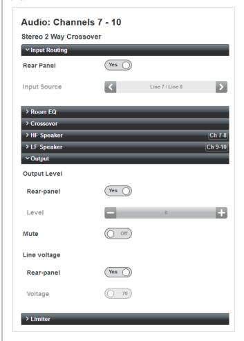
Note that the LF Speaker tab is now annotated Ch 9–10, these are in fact the two Auxiliary Outputs. In all respects, the setting-up and adjustment of the crossover is identical to that described previously, the only difference being that the two mono LF (L+R) sums will now appear at line level at the Auxiliary Outputs.
