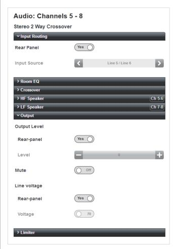
The status of the four channels is confirmed at the top of the page. Note that the HF Speaker tab is annotated Ch 5-6 but the LF Speaker tab is now annotated Ch 7-8, indicating that (in this example) Channels 7 and 8 both now form part of the crossover.
