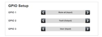
The port has three separate pins (GPIO 1, GPIO 2 and GPIO 3), each which may be configured in one of four ways – two input options and two output options. See "The GPIO Port" on page 50 for electrical and connection details of the GPIO port.
