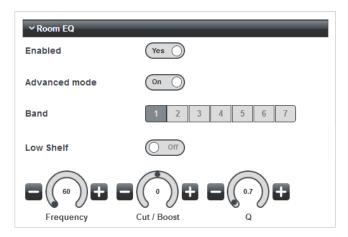
The Q control adjusts the bandwidth of the peaking filter over a range of 0.1 (broad) to 20 (narrow), with a default value of 0.7.
