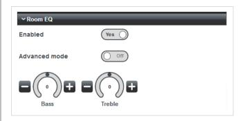
In Basic mode, simple Bass and Treble shelving filters are provided. Click the + and - buttons to adjust the EQ. The controls have a range of +/-12 dB at frequencies of 10 kHz and 50 Hz respectively.
