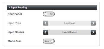
The two inputs will always be an adjacent odd/even pair, i.e., Inputs 1 & 2, 3 & 4, 5 & 6, or 7 & 8. The derived mono sum only applies to the currently-selected amplifier channel; all other channels retain the full range of inputs, including the individual odd and even inputs forming the mono sum.
