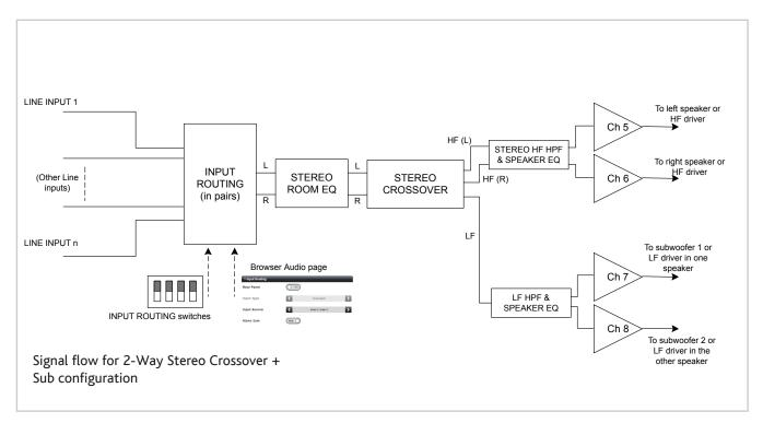
The LF components of the stereo signal are summed into a single mono signal, which to routed to the two higher-numbered channels. The HF components of the left and right input signals are routed to the two lower-numbered channels, as in the 2-Way Stereo Crossover + Mono example on page 36.
