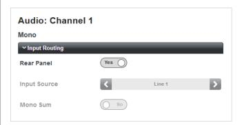
• Rear Panel – the default position for this switch is Yes. In this setting, the other controls in the tab are greyed out and input routing for the amplifier channel (or pair of channels) will be determined by the settings on the INPUT ROUTING rear panel DIP switches (see "Connections and Adjustments" on page 16). Moving the switch to No activates the on-screen controls:
