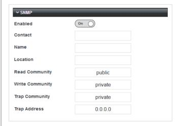
CV Digital amplifiers are compatible with system monitoring software employing the SNMP protocol. Cloud Electronics software and MIBs for the CV Digital amplifier range can be downloaded from the product page at <a href="www.cloud.co.uk">www.cloud.co.uk</a>. Once these are loaded into SNMP browser / management software, the available SNMP parameters will become available.
