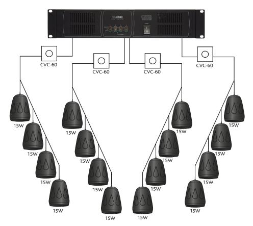
This is a simple solution where a mixer/zoner is not required. There would be only one source but the 4 spaces require independent volume control. Using a 4 channel VA4120 amplifier each channel has a CVC-60 controlling the collective volume of the 4 x CVS-P62 pendent speakers. Each speaker is tapped to 15Watts, ensuring the collective wattage dose not exceed the CVC-60 wattage limit (60Watts).
