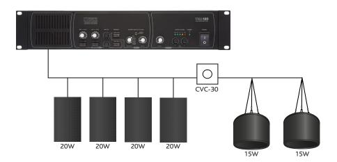
It is possible to insert a 100V attenuator anywhere along the speaker line allowing for separate volume control of the speakers post the insertion point. Again the total output of the speakers post the attenuator must not exceed the controllers wattage capability.
