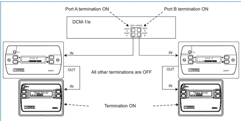
Diag. (a) shows four CDRs, each connected to one DCM-1/e port; (b) shows a single daisy-chain of two CDRs all on one port; c) shows two daisy-chains each of two CDRs using two ports. Note that in the diagrams there is deliberately no indication as to which zones any of the CDRs are in; this is because the system imposes no restriction on their physical location. CDRs in different zones may be in the same “chain”, and interconnections may be made purely on the basis of wiring convenience.
