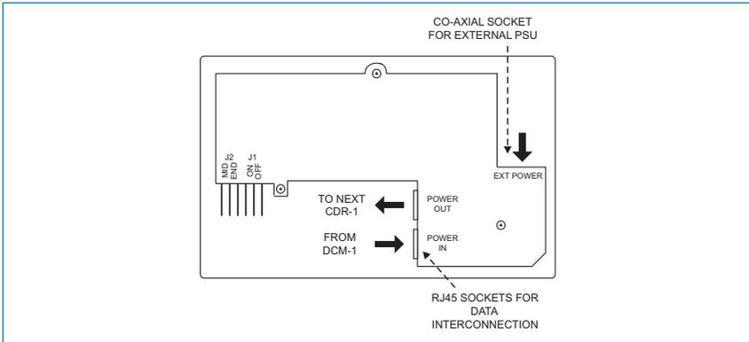
5. Check that jumper J1 is in the OFF position. J2 should be set according to the CDR-1's position in the CAT-5 "chain". If it is the final (or only) panel in the chain (i.e., nothing is plugged into the POWER OUT connector), set J2 to END; in all other cases set it to MID. Carefully use tweezers or a pair of fine-nosed pliers for this operation.
