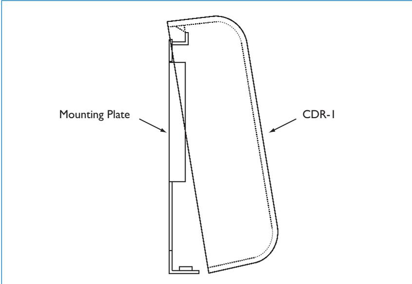
8. Screw the CDR-I to the mounting plate using the two countersunk M3 screws removed in step 1.
