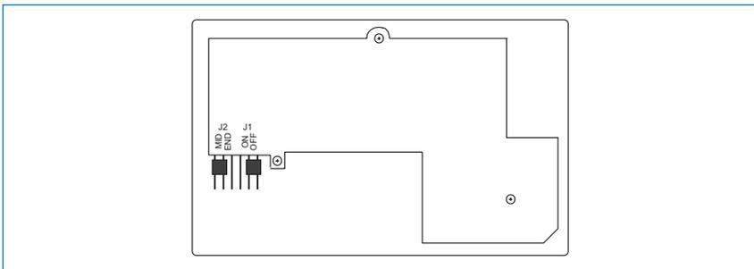
6. Angle the CDR-I so that the top is closer to the wall and push onto the mounting plate such that the two small lugs on the inside of the top of the housing mate with the corresponding flanges on the plate.
