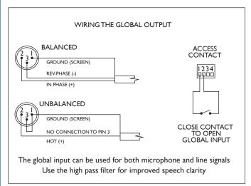
Note that if feeding the global input from an unbalanced source, pins I and 3 should be linked on the mating XLR plug as shown above.
