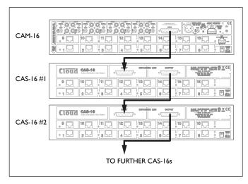
Only the multicore cable supplied with each CAS-16 should be used for interconnecting a CAM-16 and a CAS-16, or two CAS-16s. Do not attempt to locate a CAS-16 remotely from its CAM-16 base unit, or from other CAS-16s in the system, by the use of a longer cable.
