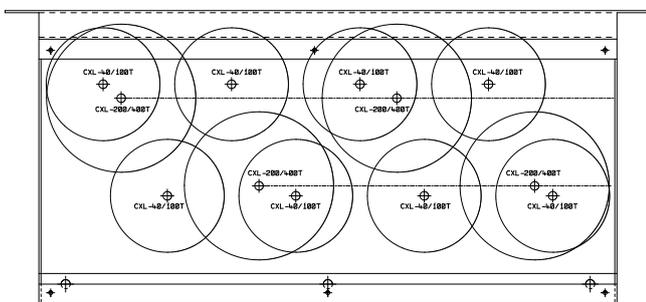
When each transformer position has been determined, insert the bolt from the underside of the chassis, place the transformer in position with the bolt through the central hole, and secure it in place with the washer and locknut supplied. Before final tightening, rotate the toroids to ensure that the cable assemblies for all the transformers emerge from the windings at a neat orientation for wiring to the rear panel.
