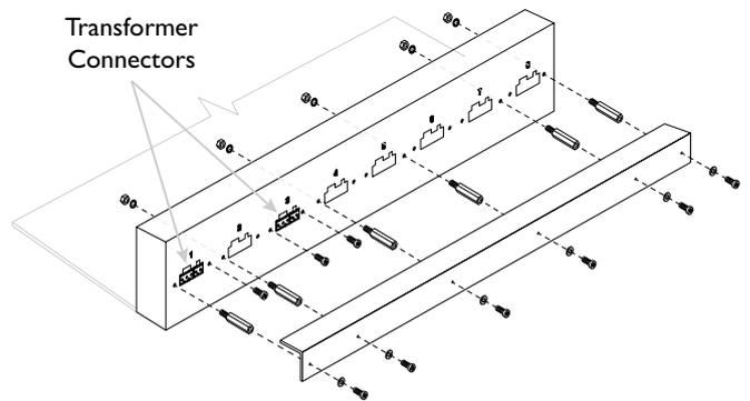
**IMPORTANT:** If less than eight transformers are installed in the rackmount housing, it is still important to fit all six hex pillars (supplied) in the positions indicated. If a connector position requiring a hex pillar is empty (due there being no transformer in that position), use an M3 shakeproof washer and nut (supplied) to secure the hex pillar in place.
