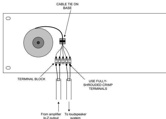
If transformers are being freely-mounted on a panel within an equipment rack, fit lockable side and rear doors, and blank 19” panels as necessary to the rack, to prevent access to the terminations. If the transformers are to be housed externally to a rack, the use of a lockable IP-rated enclosure fitted with the appropriate cable grommets is recommended.
