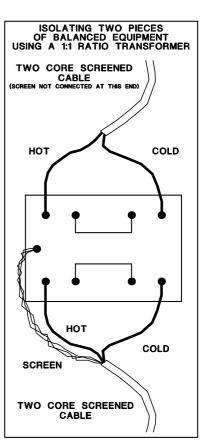
AUDIO TRANSFORMER RS PART NUMBER: 210-6447 FITTED WITH SCREENING CAN RS PART NUMBER: 210-6469
